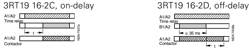
Fig. 3-56: Solid-state time relay block with semiconductor output, function diagrams (frame size S00)
